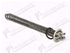
Resistenza boiler 9000W 230V L=475 mm; flangia Ø 64 mm; Øint. 50 mm; guaina portabulbo 2 x L=195 mm; O-ring 5,34x46,99 mm
