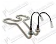
Resistenza vasca 2000W 230V dim. 200x135 mm; faston F6,3 mm; faston F Ø 2 mm; cavi L=160 mm
